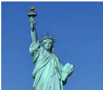
According to the National Park Service, the Statue of Liberty contains 31 tons of copper 3/32 inches thick.
